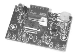
● CAUTION. The TD-5 contains static sensitive ic's, which require normal static prevention techniques when handling to avoid damage. Wearing a grounded wrist strap is a prudent practice. For wired units, do not remove the unit from its protective package until ready to install. For kits, do not open package with semiconductors until ready to install on board.
