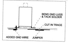
c. Looking under the board, you will note that one ground lug of each coil was meant to carry the ground connection through the board to provide grounds for other components. These are the lug holes closest to the right side of the board. Because the ground lugs of the new shield cans are tack soldered on the top of the board instead, it is necessary to run a short length of #22 bus wire through these holes, soldering both the
