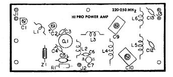
Hi Pro PAV 1 Power Amplifier 222MHz
