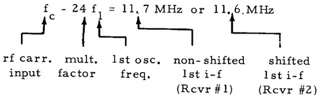
NOTE: If a shift of high i-f frequency is required in a two-receiver station, it will be the higher (rf) frequency receiver whose i-f frequency is shifted from 11.7 to 11.6 MHz.
