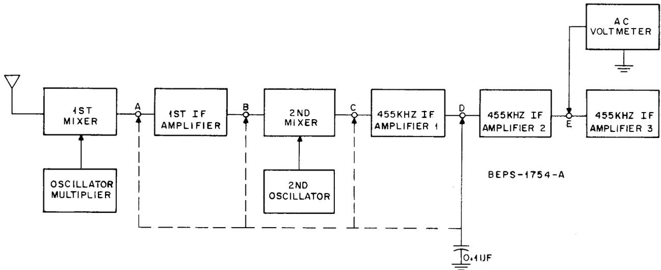
Figure 3. "Noise Gain" Measurement Test Set-Up
