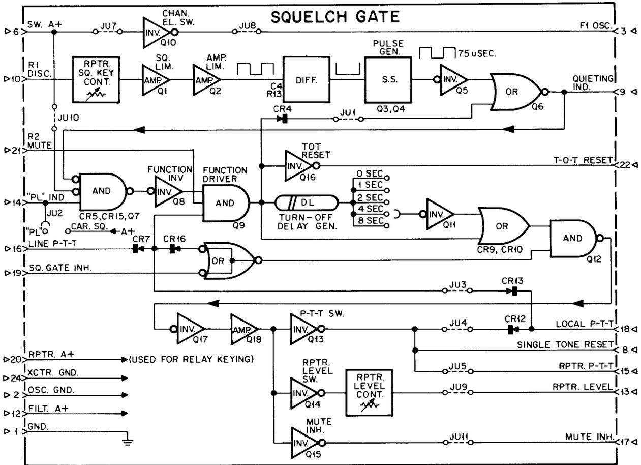
A LOW AT THE INPUT OF THE DELAY GENERATOR IS DELAYED AT THE OUTPUT OF Q11 BY THE TIME SELECTED BY THE TAPS.
