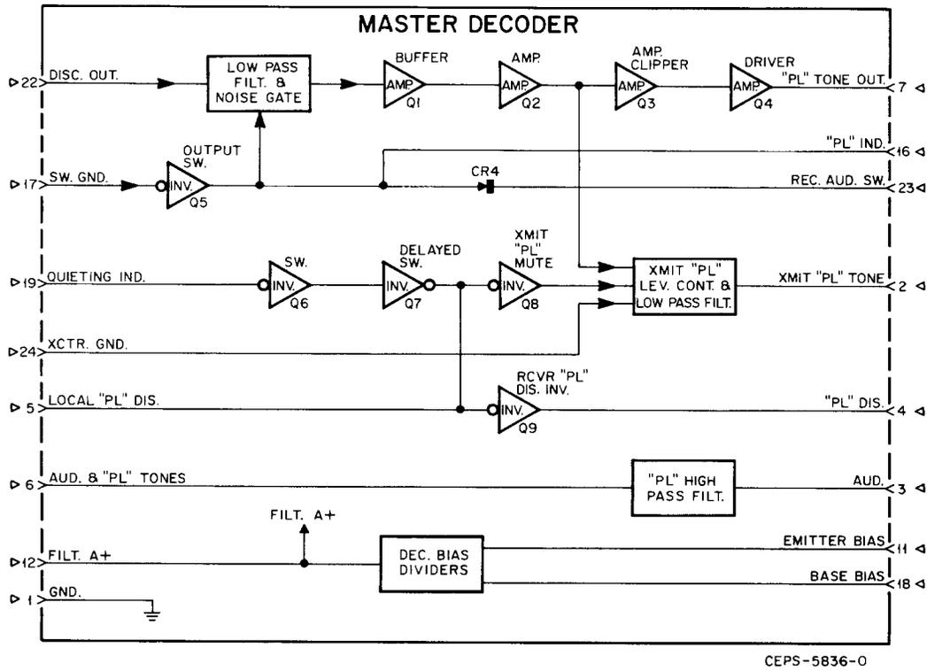
Master Decoder Module Functional Block Diagram
