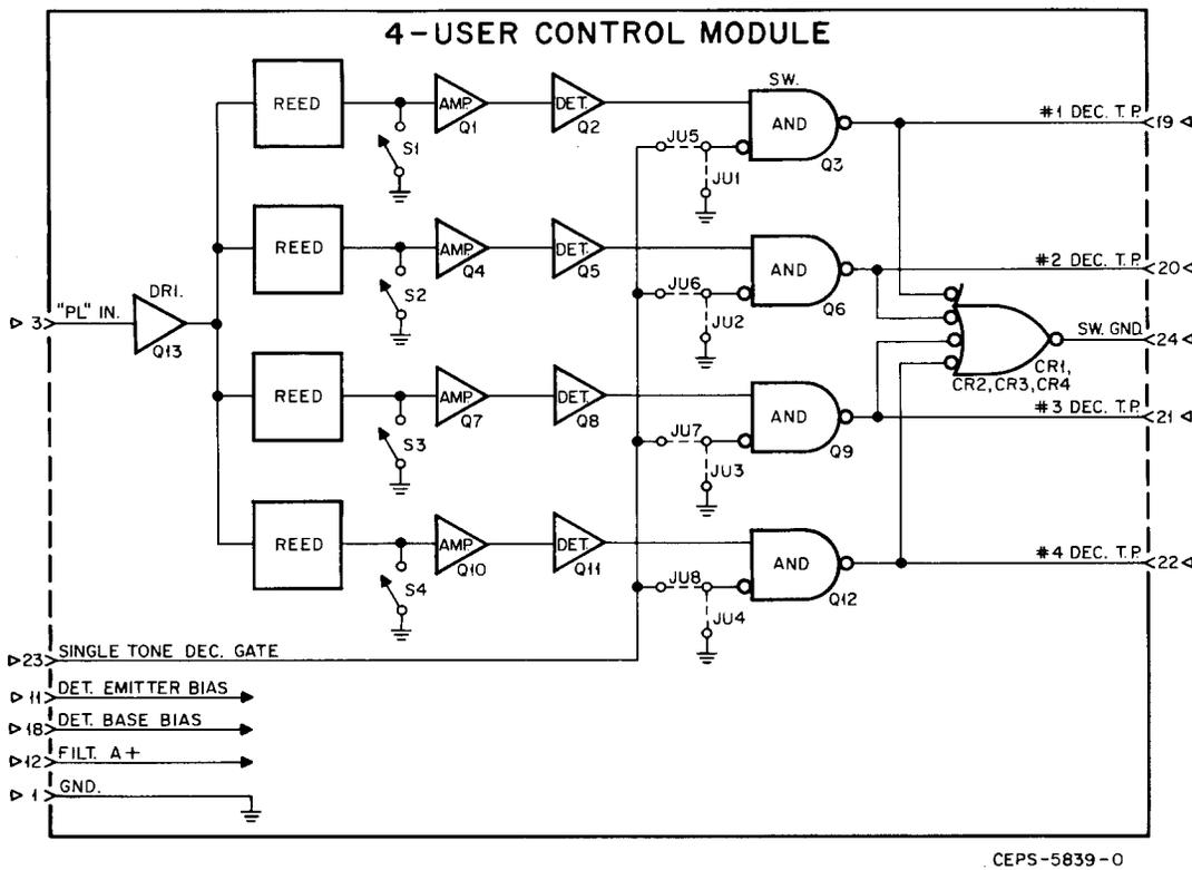
4-User Control Module Functional Block Diagram
