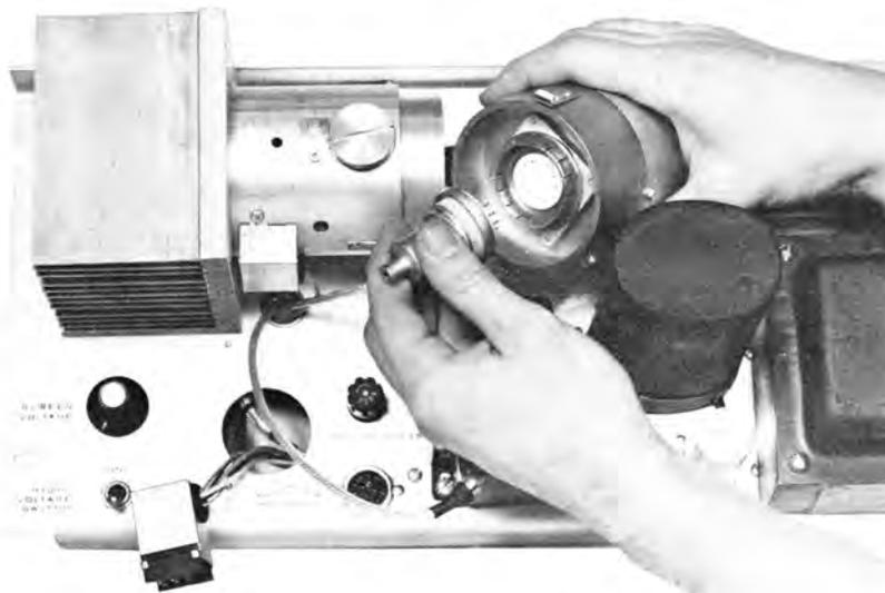
Power Amplifier Tube Removal Detail B
