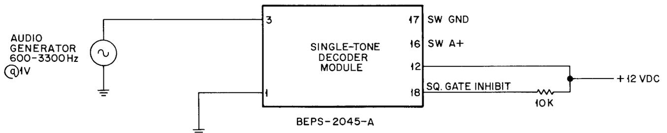
Test Set Up Diagram
