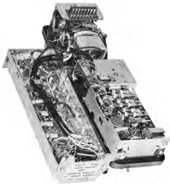
Figure 3. Receiver in Service Position
