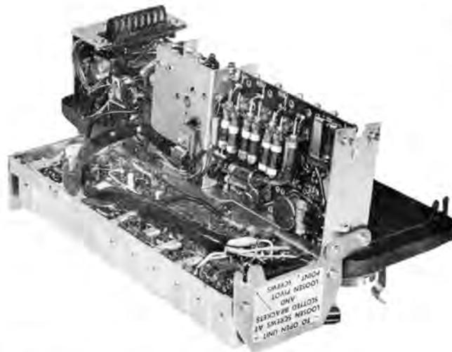
Figure 4. Transmitter in Service Position
