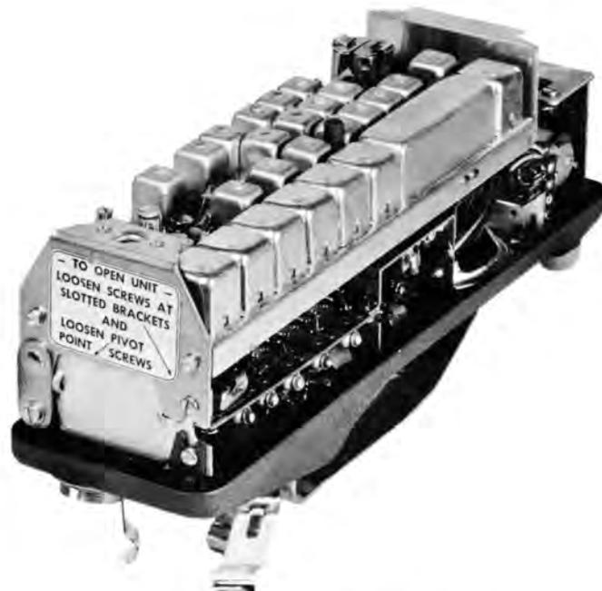
Figure 2. Radio Section Exposed
