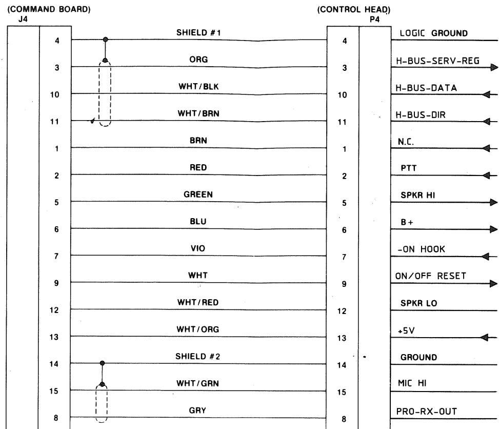
\* CABLE PIN ASSIGNMENTS ARE FOR PARALLEL CONTROL HEAD.
