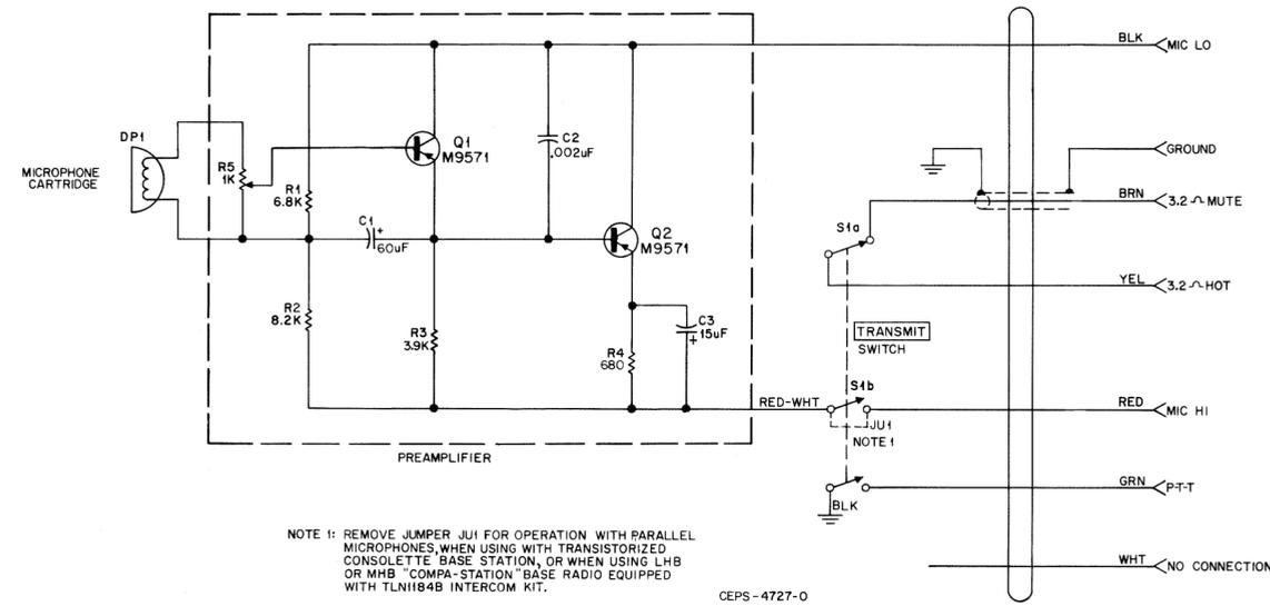
NOTE 1: REMOVE JUMPER JU1 FOR OPERATION WITH PARALLEL MICROPHONES WHEN USING WITH TRANSISTORIZED CONSOLETTA BASE STATION, OR WHEN USING LHB OR MHB "COMPA-STATION" BASE RADIO EQUIPPED WITH TLN1848 INTERCOM KIT.
