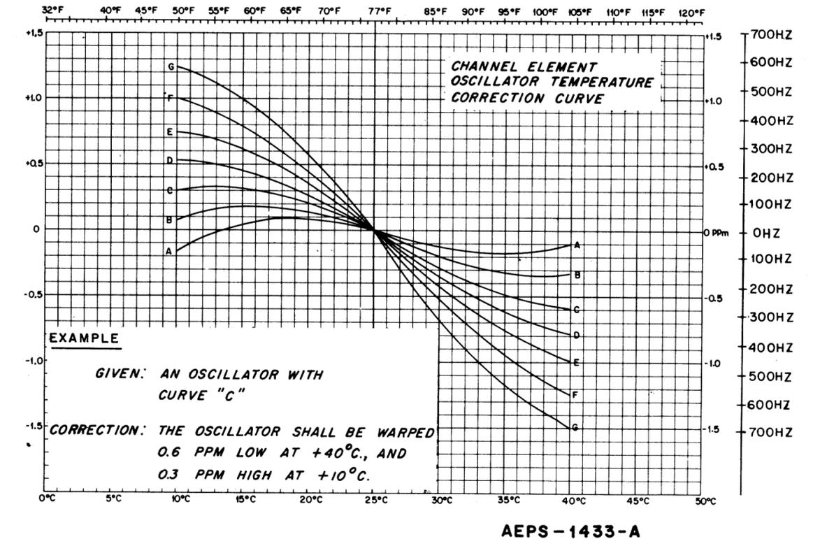
Oscillator Temperature Correction Curve
