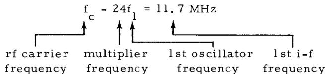
e. First Intermediate Frequency (High IF) Circuit
