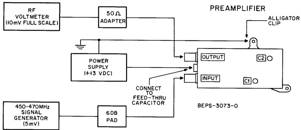
3. Motorola Model TEK-23 Regulated Power Supply, or equivalent.
