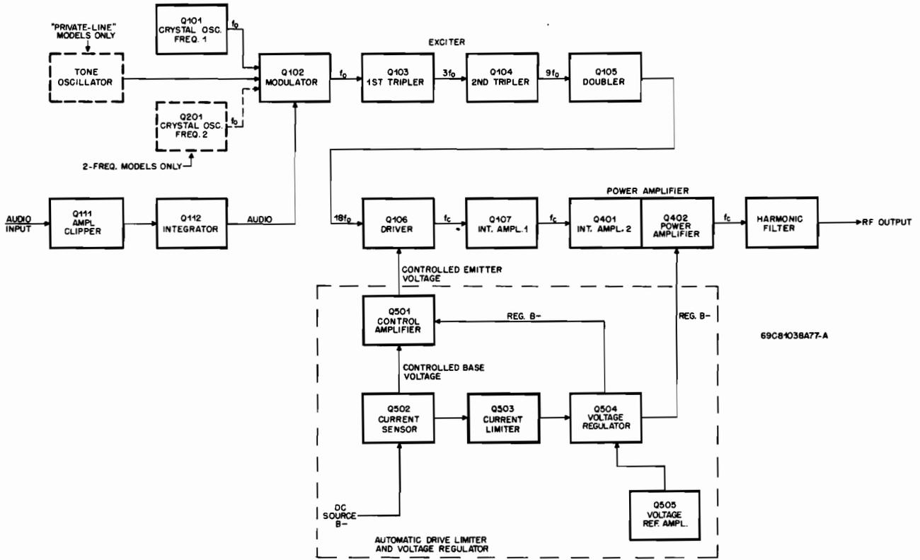
Transmitter Block Diagram
