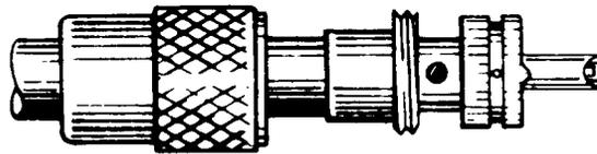
SCREW THE PLUG SUB-ASSEMBLY ON CABLE. SOLDER ASSEMBLY TO BRAID THROUGH SOLDER HOLES.
