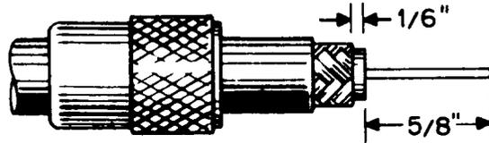
BARE 5/8" OF CENTER CONDUCTOR. TRIM BRAIDED SHIELD. SLIDE COUPLING RING ON CABLE. TIN EXPOSED CENTER CONDUCTOR AND BRAID.
