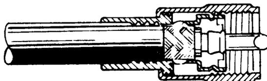
FOR FINAL ASSEMBLY, SCREW COUPLING RING ON PLUG SUB-ASSEMBLY.
