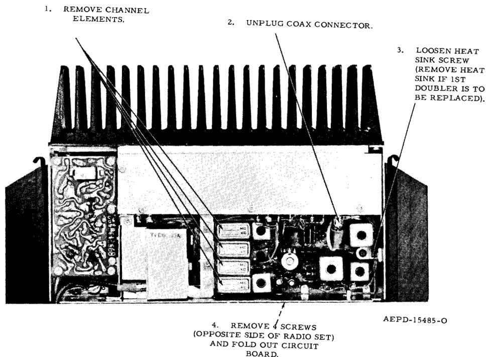
Figure 32. Access to Exciter Components
