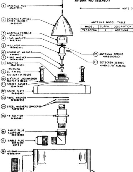
NOTE: ITEMS 1 TO 7, 20&21 CAN BE OBTAINED PRE-ASSEMBLED (PART NO. 1B 893662 ANTENNA ROD ASSEMBLY)
