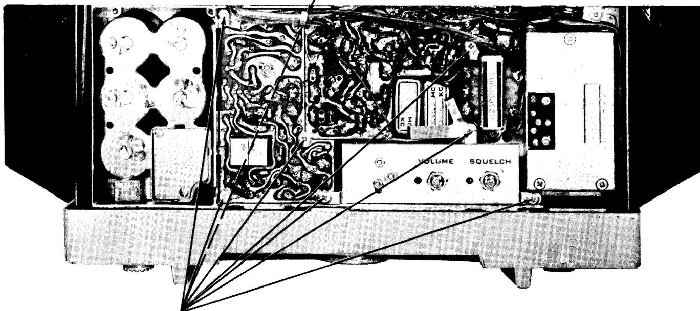
2. REMOVE MOUNTING SCREWS AND CAREFULLY FOLD OUT BOTH BOARDS TOGETHER. ALSO FOLD OUT VOLUME AND SQUELCH DECK. USED CARE WHEN FOLDING OUT BOARDS TO ASSURE INTERCONNECTING LEADS ARE NOT BROKEN.
