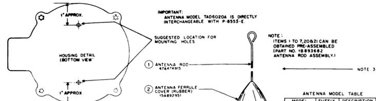
IMPORTANT: ANTENNA MODEL TAD6020A IS DIRECTLY INTERCHANGEABLE WITH P-8555-E
