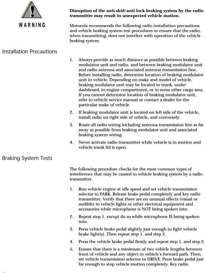
transmitter. Verify that vehicle does not start to move while microphone is NOT being spoken into.
