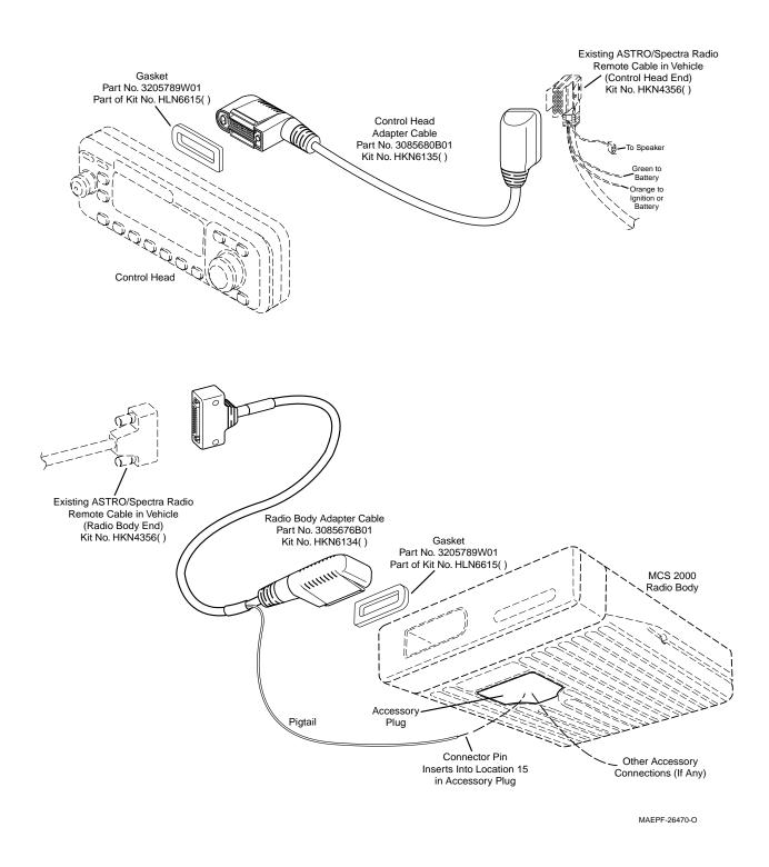
Figure 1 ASTRO/Spectra to MCS 2000 Adapter Cable Set
