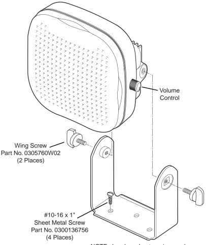
NOTE: Loudspeaker trunnion can be mounted either upright or upside down.
