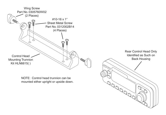
Figure 1 Mounting Rear Control Head
