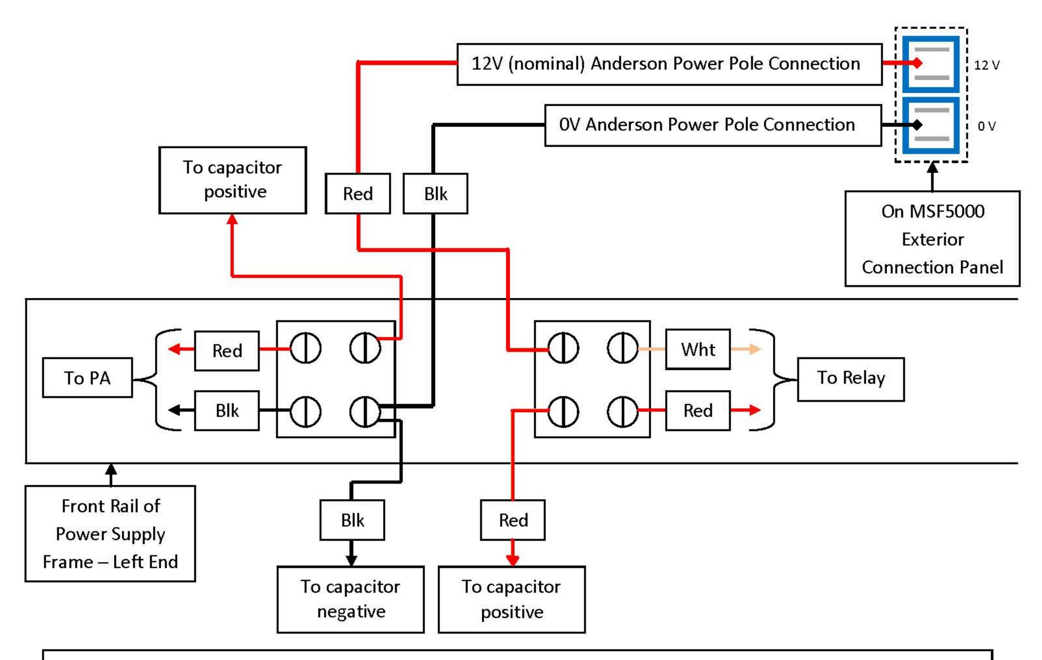
All voltages are nominal and the actual voltage could be higher or lower, depending on the type of battery used.
