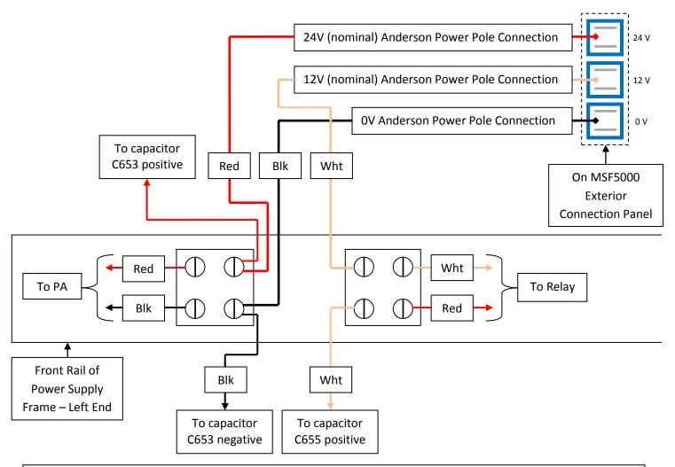
All voltages are nominal and the actual voltage could be higher or lower, depending on the type of battery used.
