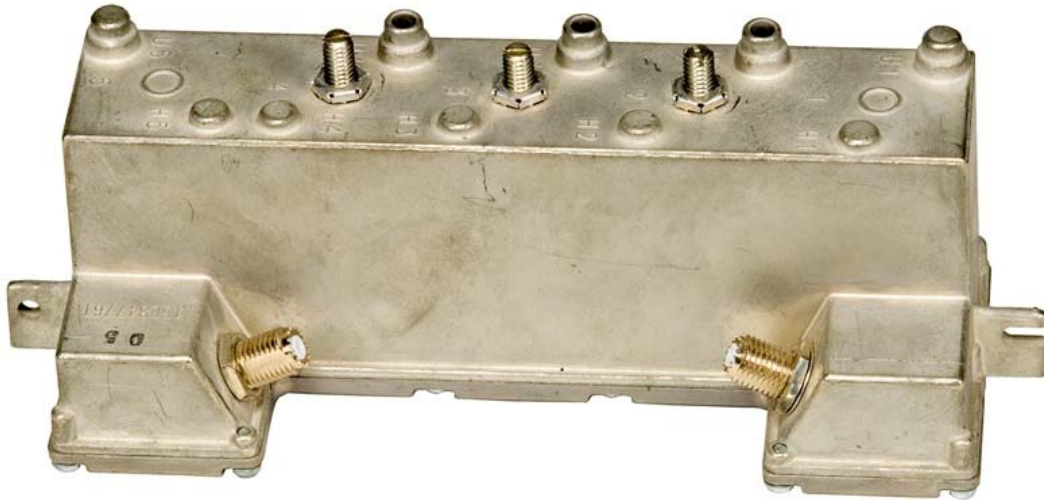
Figure 12. UHF Base Station/Repeater Preselector
