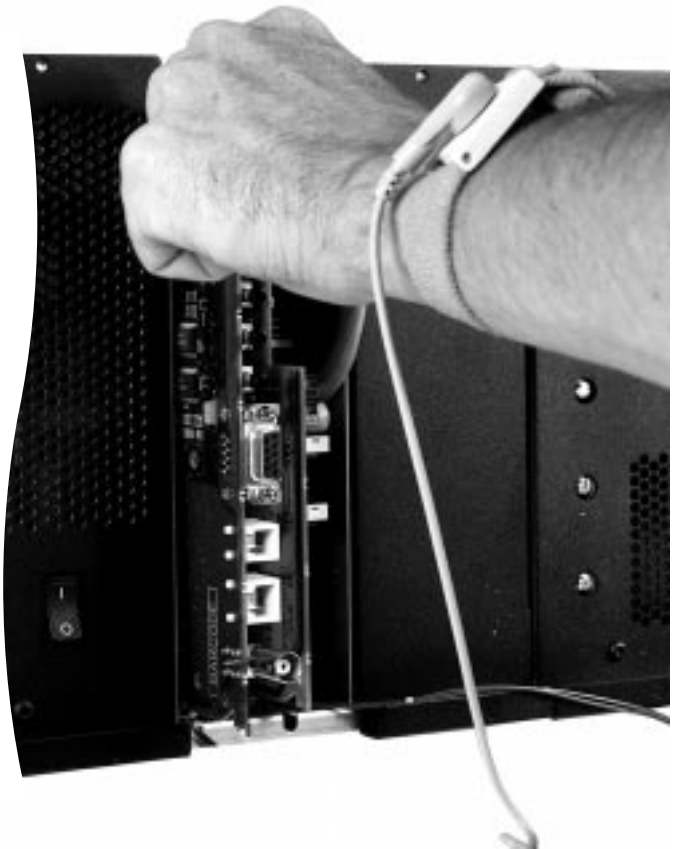
Figure 6. Removal Procedure for Station Control Board (Quantar VHF Station Shown)
