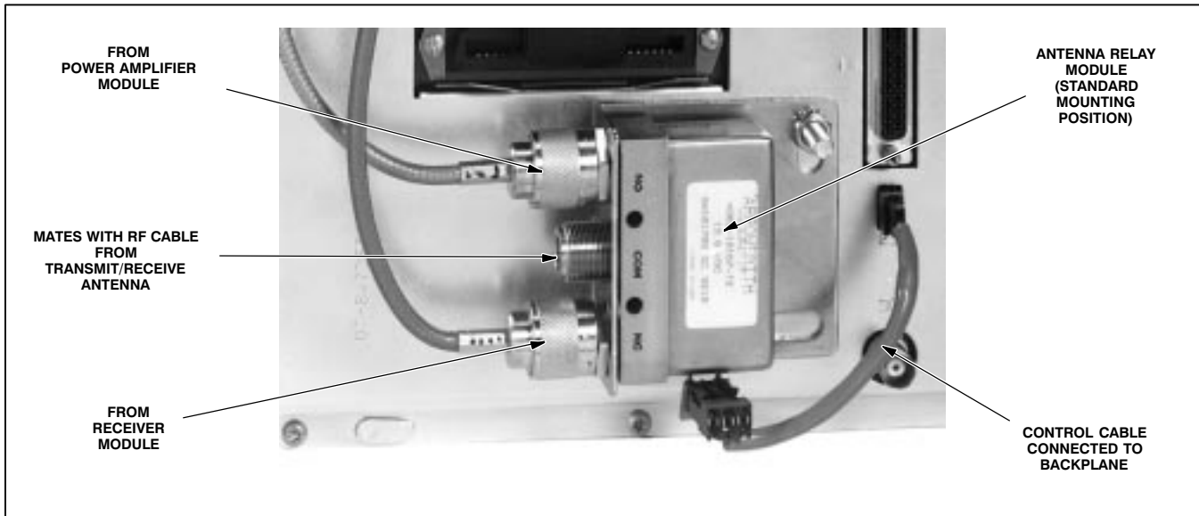
Figure 3. Standard Mounting Position for Antenna Relay Module
