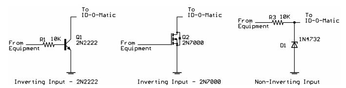
The Connection Kit can make connecting your ID-O-Matic to other equipment much easier. It provides inverting and noninverting inputs, voltage limiting, an audio amp/mixer/filter, and optional PTT for many handheld transceivers. It is designed to plug directly onto the ID-O-Matic board "piggy-back" style. You can check out the Connection Kit at HamGadgets.com.
