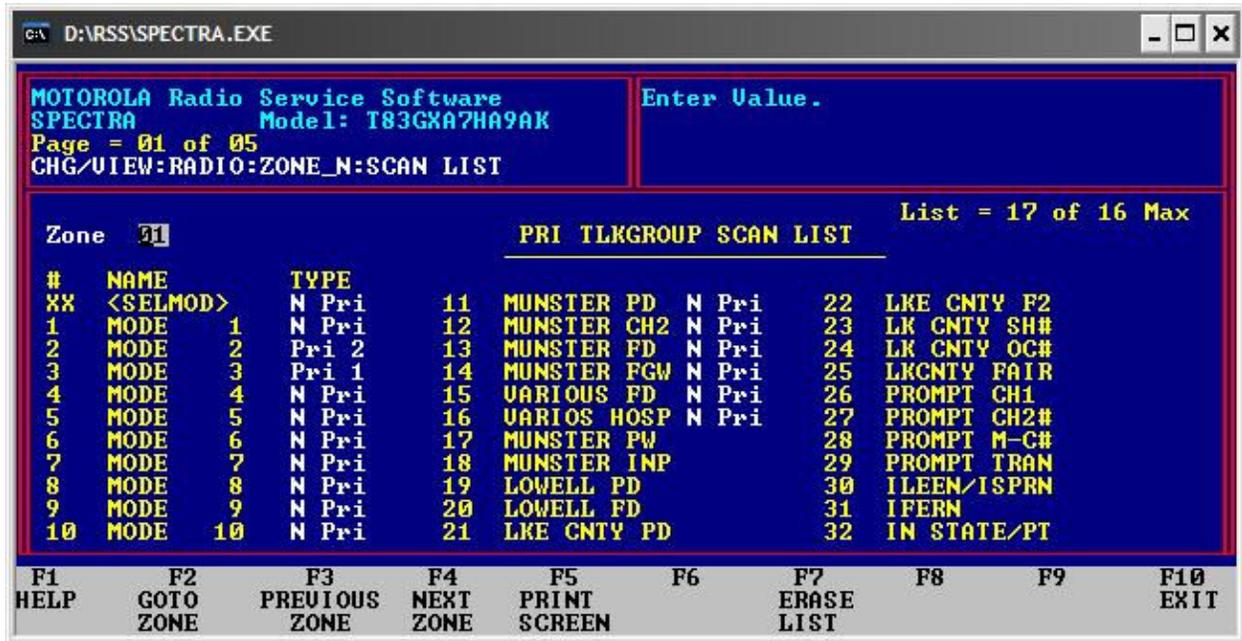
Now, it reads "17 of 16 Max". Go ahead and add more modes to scan. Just be sure to NEVER DROP IT TO 16 OR BELOW. If you do, you will have to repeat the process. Here is an example of an exceeded scan list! 😊
