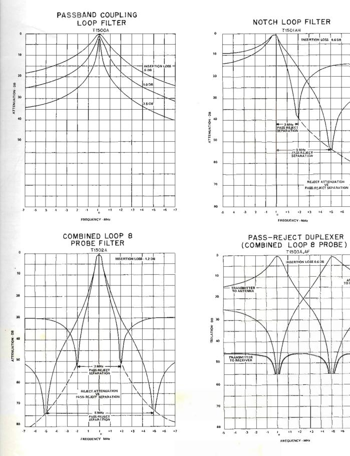
Figure 15. Filter and Duplexer Selectivity Curves Typical for 430-470 MHz Range
