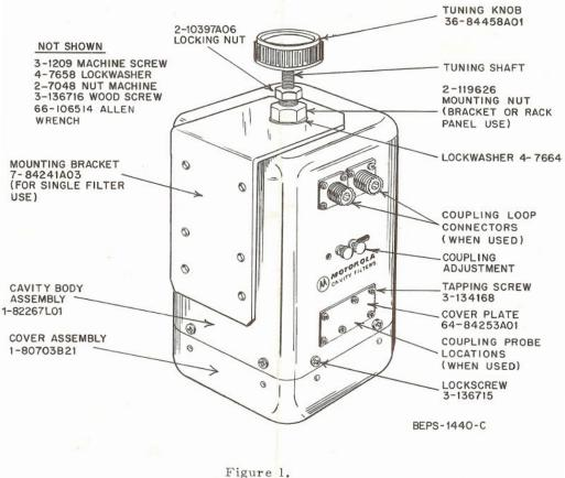
Cavity Filter Parts Location Detail
