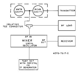
Figure 13. Method 2 Receiver Branch Reject Test Set-Up
