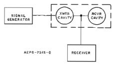
Figure 11. Method 2 Transmitter Branch Reject Test Set-Up
