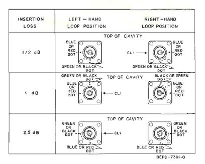
Figure 5. Coupling Loop Positions (Exterior View)
