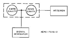
Figure 12. Method 2 Receiver Branch Pass Test Set-Up
