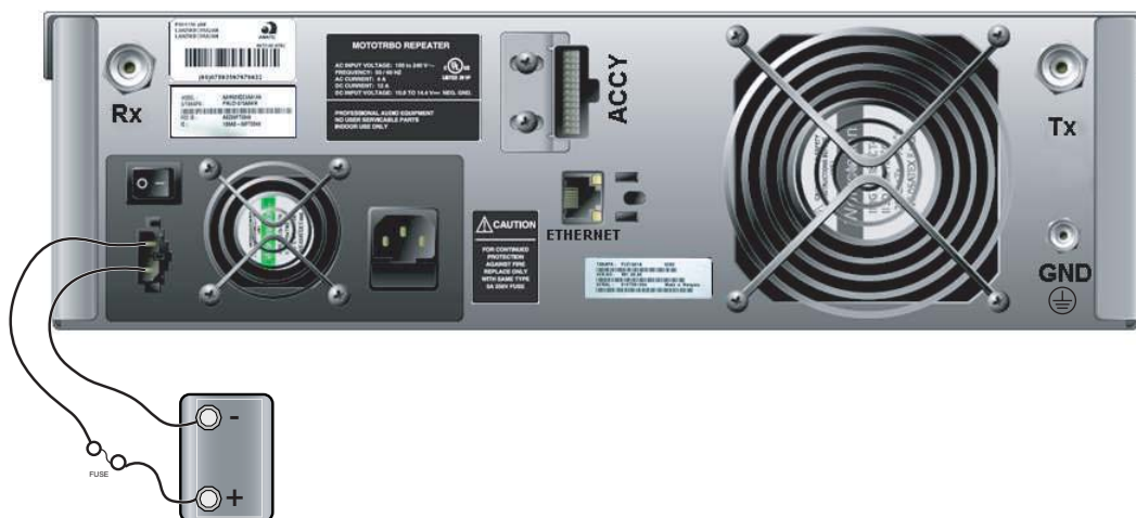
Figure 4-2 Making Connections to a Backup Battery
