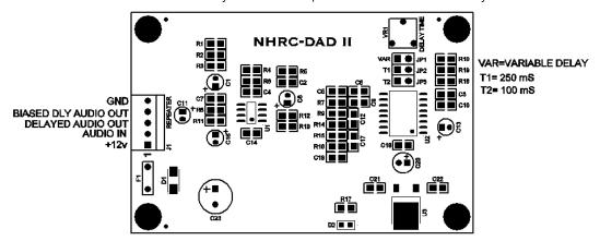
The AC coupled audio input impedance is approx 100K ohms. Max audio input is 2V P-P. Audio output impedance is approx. 70 ohms and is user selectable DC biased or AC coupled output. DC biased output is required on all NHRC controllers. An AC coupled output is provided for use with controllers of other manufacturers. DC input requirements: 9-16v 25mA
