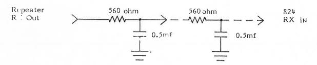
This circuit can be cascaded for further attenuation.
