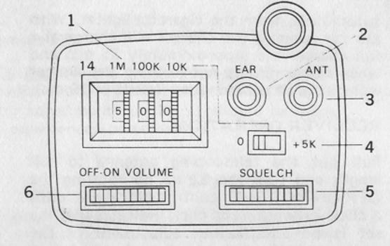
Thumbwheel switches for selection of MHz, 100 KHz, and 10 KHz.
