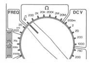
3. Connect the probes to the diode you want to check and note the meter reading.
