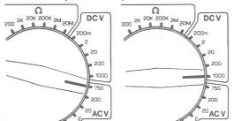
Select the range as required for the voltage level to be measured. If you do not know the voltage level, start with the range switch set to the highest voltage position and reduce the setting as needed to get a reading.
