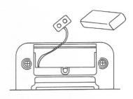
Replace the battery compartment cov and the screw. WARNING: DO NOT OPERATE THE METER UNTIL YOU REPLACE THE BATTERY AND CLOSE THE BATTERY COMPARTMENT COVER.
