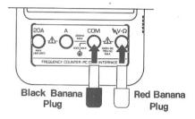
Connect the black probe to the ground point (GND) of the test circuit and the red probe to the supplying voltage point (V+). While keeping the test probes firmly connected to each point, press LOGIC REL.
