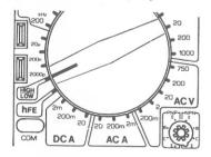
2. Plug the black probe into your meter's **COM** terminal and the red probe into your meter's  $V \cdot \Omega$  terminal.
