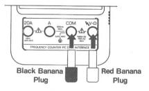
3. Connect the probe to the frequency source.
