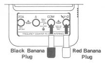
3. Connect the probes to the AC/DC voltage source you want to measure.
