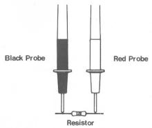
**Note:** The buzzer sounds if the measured resistance is below 30 ohms.
