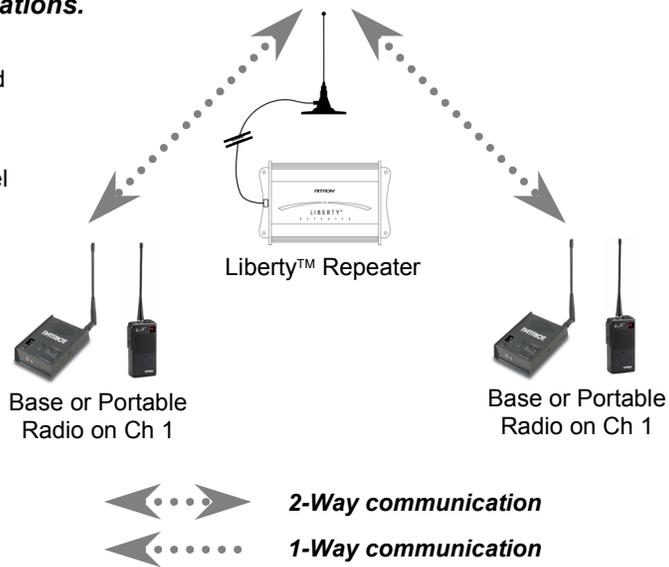
The Liberty™ Repeater and especially the installation location of its antenna are the most important pieces of your system. The location of the antenna is critical to achieving optimal radio coverage. When properly installed and connected to the Ritron Liberty™ Radio Repeater, you will be able to extend the range and coverage of your Liberty programmed 2-way radios\*.
