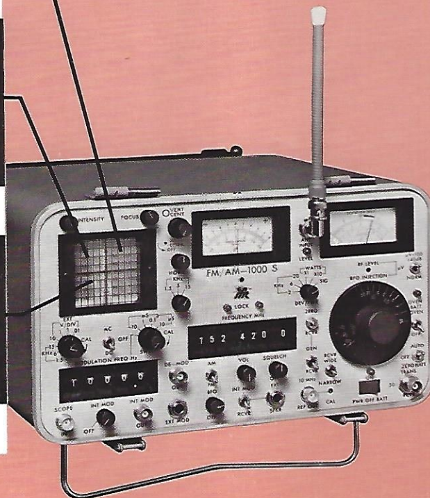
NARROW DISPERSION: Analyzer sweeps \pm 0.5 MHz from selected frequency (1 MHz span)
