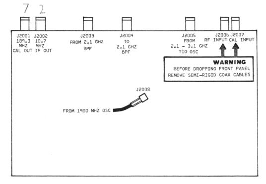
Figure 4-2. RF Casting Cable Connection Locations
