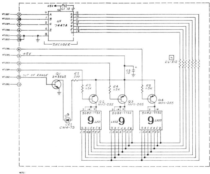
1. RESISTORS - 1/4W. 5% VALUES IN OHMS UNLESS OTHERWISE NOTED. 2. CAPACITORS - VALUES IN  $\mu$ F UNLESS OTHERWISE NOTED. 3. INCUCTORS - VALUES IN  $\mu$ H UNLESS OTHERWISE NOTED. 4. \*\*RACTORY SELECT. TYPICAL VALUE SHOWN. 5. ALL VOLTAGES ARE DC UNLESS OTHERWISE NOTED.
