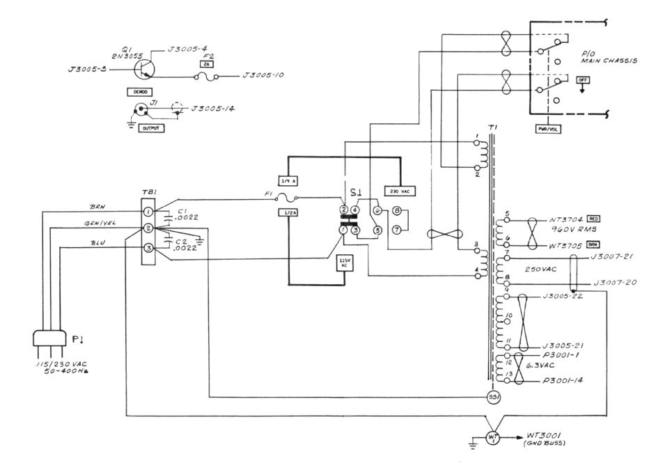
Figure 5-18. Rear Panel Interconnection Diagram, 4000
