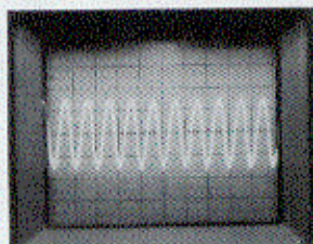
Photo 2 Pin 1 of P1 Tone decoder input RFSG to Rx Ant. Level: 1000 uV Dev: 500 Hz Mod. Freq: 150 Hz Scale H: 5ms/Div V: 50mV/Div DCV: 1V
