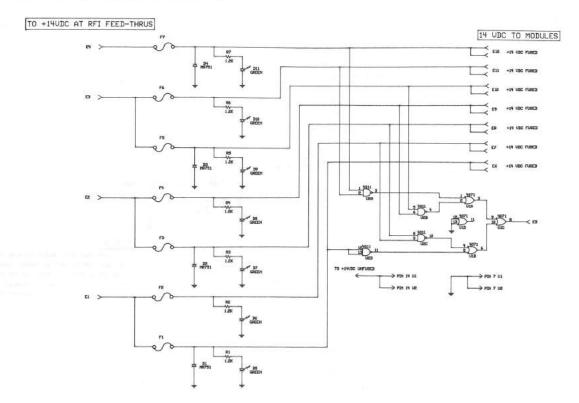
The DC distribution board serves several functions. It provides a termination point for the incoming high current DC voltage, a convenient mounting for the DC power line fuses, a mounting for the reverse protection diodes, and a distribution point for DC power to the modular subassemblies.
