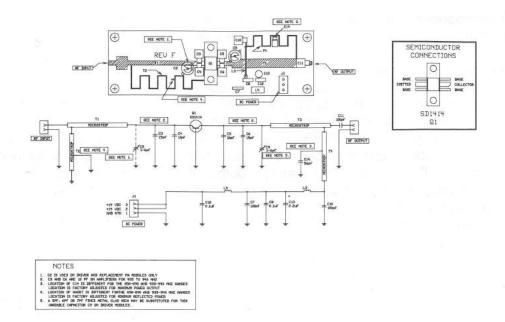
This module is common to all 14 V, 900 MHz RF power amplifiers and is used as a driver and final amplifier. The driver module and replacement final amplifier modules include a variable capacitor C15 on the base for minimizing the input VSWR.
