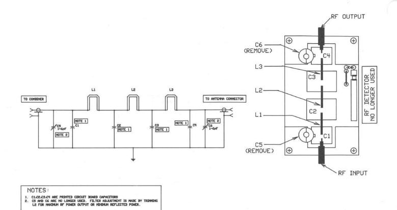
The seven pole, low pass filter is a CHEBYCHEV 0.1 dB ripple design. The filter reduces all harmonics by a minimum of 35 dB.
