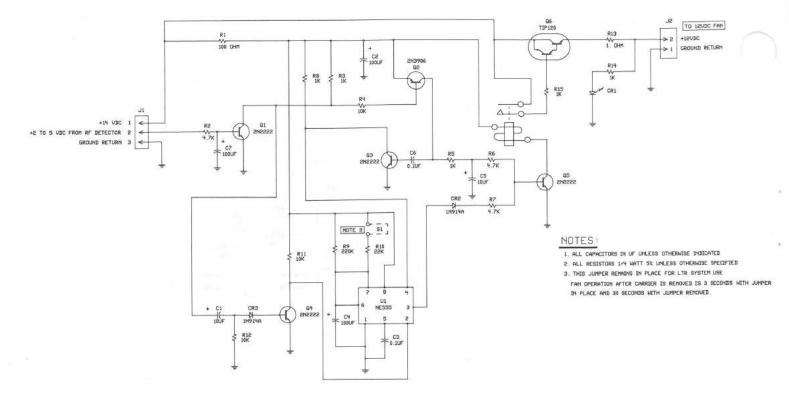
RF power controls the fan in the ARX 1200/1200A/1600 continuous duty amplifiers. A 555 timer and supporting circuitry activates the fan when the amplifier is turned on.
