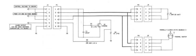
This module reduces the power output of the amplifier if the heatsink temperature rises above 135°F. When the temperature drops below 115°F, the power is again restored to its original level. When an over temperature occurs, a +12 VDC signal appears on a feed-thru terminal for use in actuating external alarm devices of the customer's choosing or MILCOM ALARM CONTROL MODULE #540-085.
