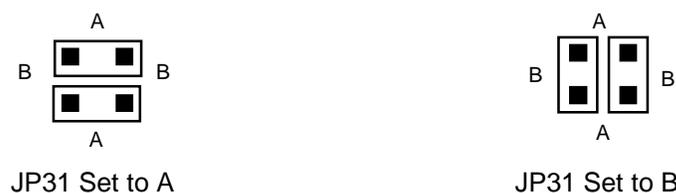
**Figure 6. INSTALLATION-3 Jumper JP31 Settings**
