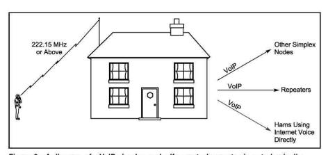
Figure 2—A diagram of a VoIP simplex node. If a control operator is not physically present at the station location and the node is functioning with wireless remote control, the control link must operate above 222.15 MHz. See the sidebar, "Is It Legal?".
